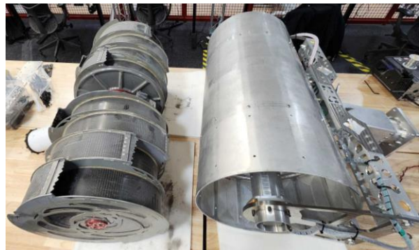
Figure 2. RASSOR excavator bucket drum (left) and TRL 4 STOMP vibratory roller compactor (right).
